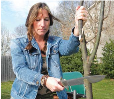
The author's wife, Melissa, chopped 2-inch-diameter tree branches using the McInnis Big Chopper (above) and Bullard Rustic Bowie (below), getting more than halfway through each branch on the first chop, and all the way through in two or three chops.
