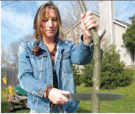
The author's wife, Melissa, chopped 2-inch-diameter tree branches using the McInnis Big Chopper (above) and Bullard Rustic Bowie (below), getting more than halfway through each branch on the first chop, and all the way through in two or three chops.
