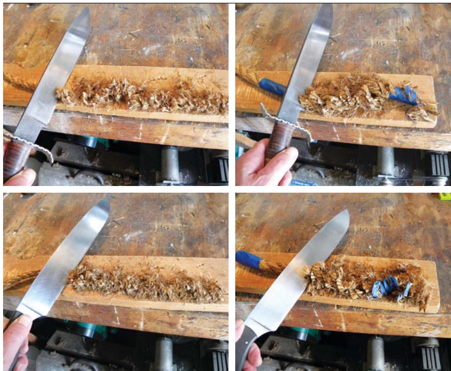
The evenly matched Rustic Bowie (top) and Big Chopper (bottom) each reached 100 crunching cuts through ½-inch sisal rope and 20 cuts through 1-inch manila rope, with both edges retaining their sharpness after testing.
